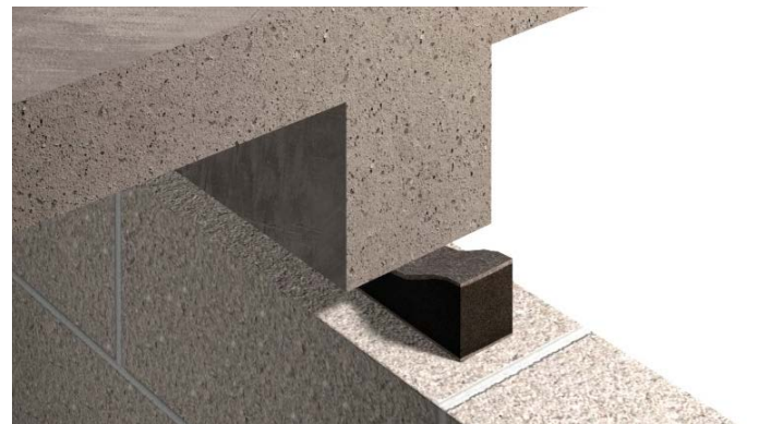
QI Intufoam Linear Joint Seal installed as a head of wall detail
