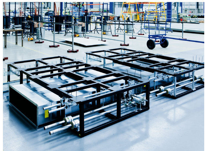
Figure 4 Example of a prefabricated corridor M&E module
