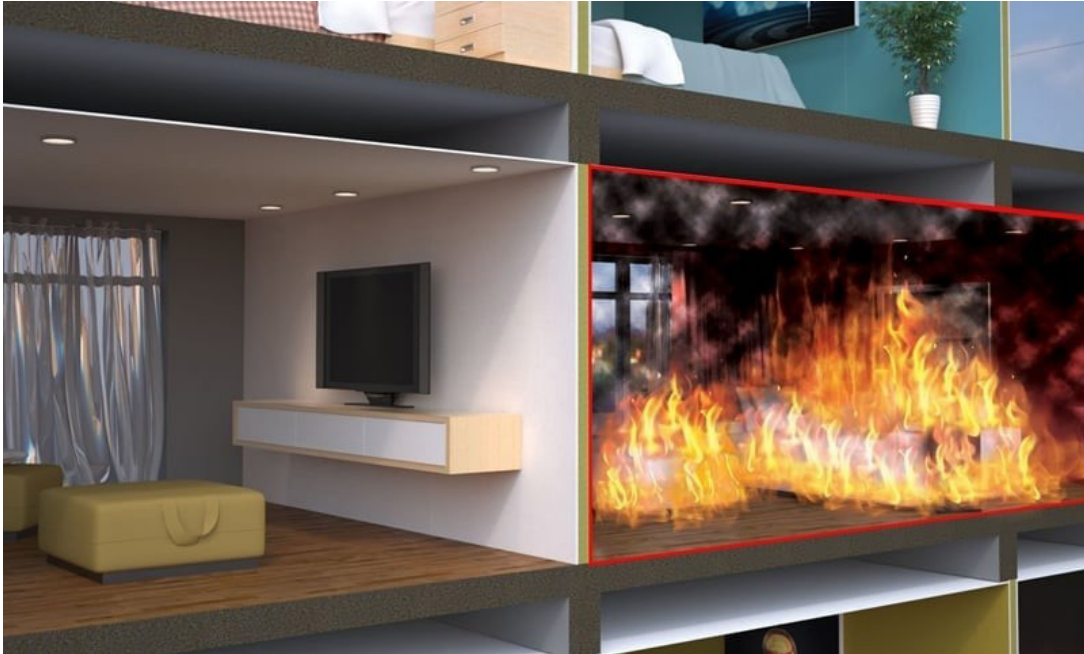
Figure 1 Compartment walls and floors between dwellings
